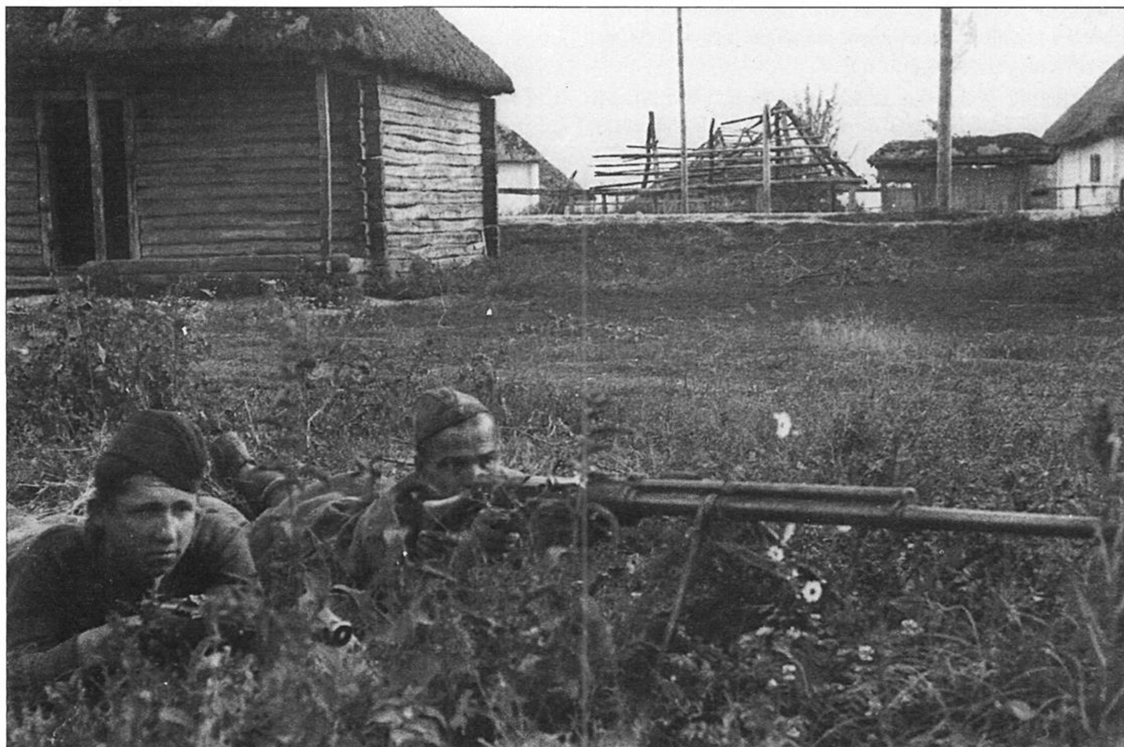
Above: A Soviet 14.5mm (0.6in) Simonov PTRS 1941 antitank rifle crew. The PTRS 1941 was a gas-operated rifle with a five round magazine; it was heavier and more complex than the PTRD but could penetrate 25mm (1in) of armour at 500 metres (546 yards).
