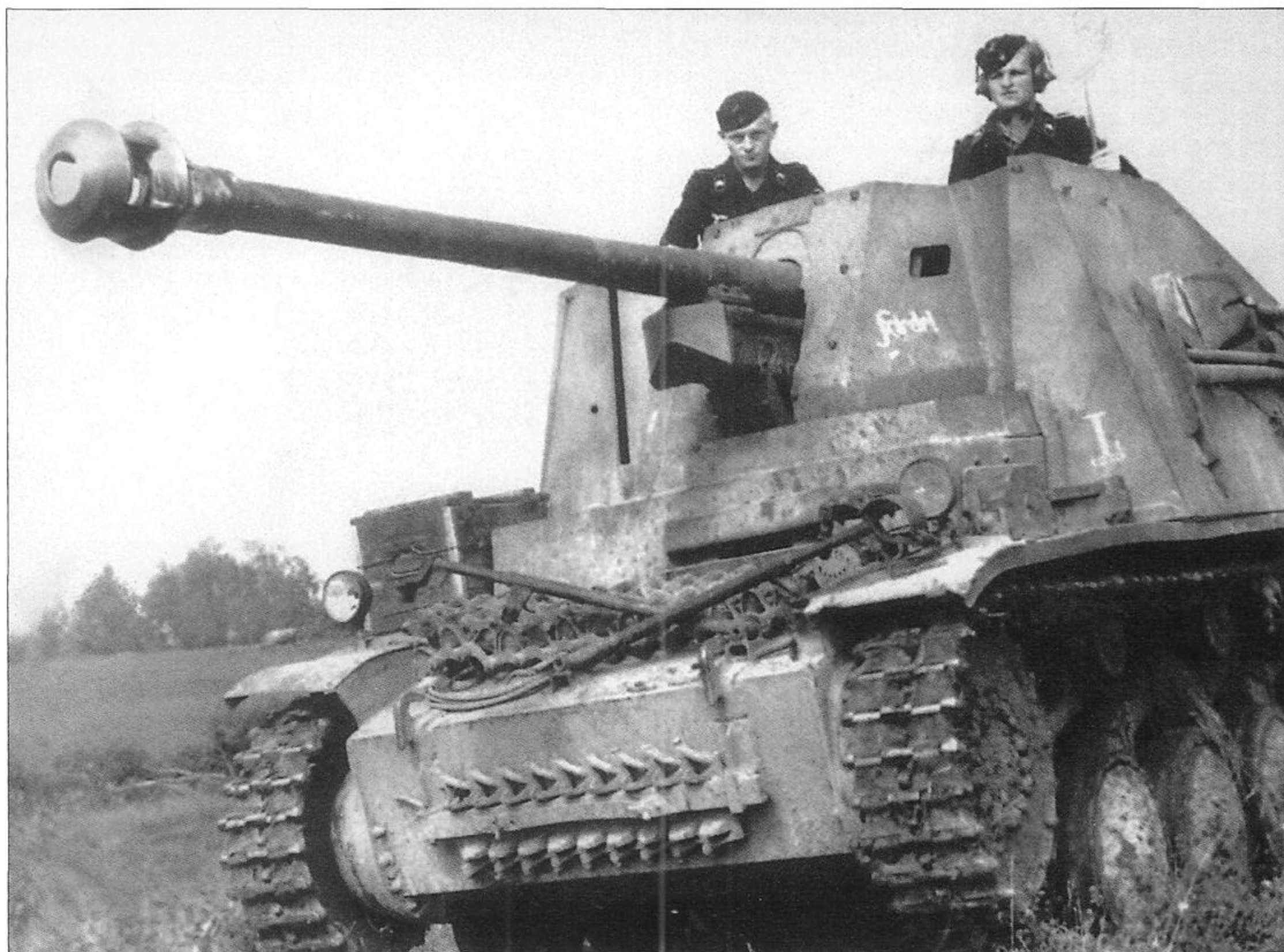
Above: A 7.5cm (3in) Pak 40/2 auf Sfl II Marder II Sdkfz 131 self-propelled antitank gun. Mounted on a PzKpfw II chassis, the gun had a maximum range of 1.8km (1.1 miles); firing AP40 shot from 500m (546yds), it could penetrate 115mm (0.5in) of armour at 30 degrees.
